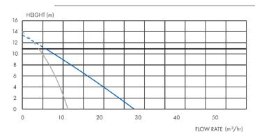
Sanipump (bladed) Sanipump (vortex)
